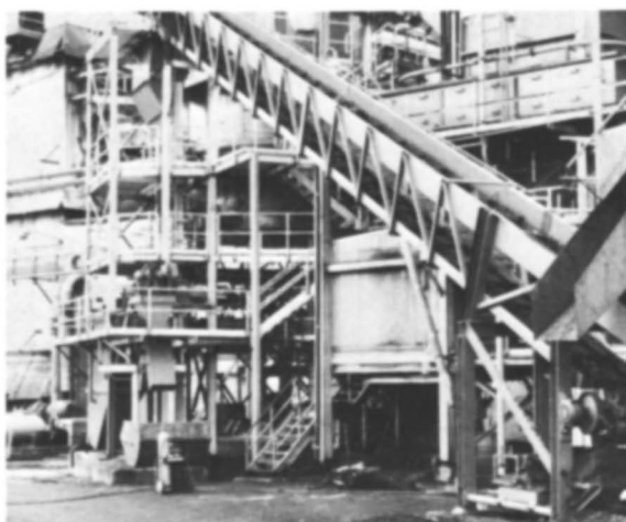
Figure 4. View and schematic of FBC hog fuel drying installation
