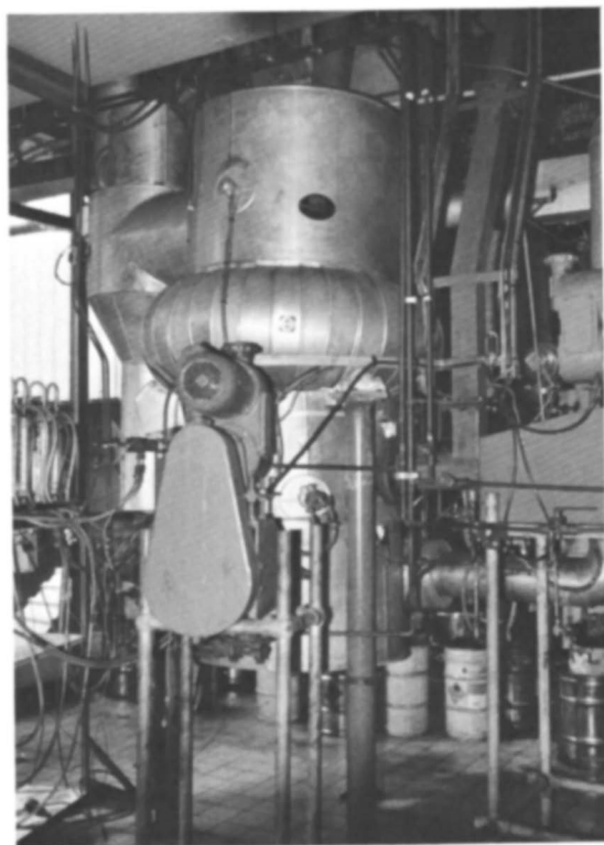
Figure 4. Pyrolysis reactor with a feed screw for plastic, a withdrawal screw for solid materials, and a cyclone
