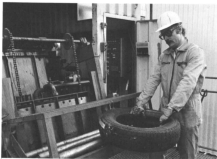
Figure 7. Placement of whole tires into the lock of the prototype reactor
